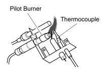
Figure 40 - Incorrect Pilot Flame Pattern
